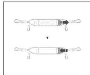
The VOLT work seat comes with two quick links and is installed via specifically-designed slots on the sides of the harness, for better load distribution between the waistbelt and the work seat.
